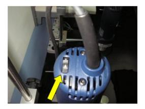
The speed is selected by the control knob on the top of the drive. Approximate rpm of the drive is: A= 10,000 rpm B= 12,000 rpm C= 15,000 rpm, D= 18,000 rpm E= 22,000 rpm F= 25,000 rpm, G=30,000 rpm
