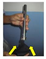
Use a piece of cloth to hold the stator as the teeth are sharp and can cut you! While holding the stator turn the shaft tube clockwise!
