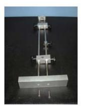
Once this bottom "H" has been fixed, take the double rod and insert into the middle piece of the foot stand. Turn it around and fix it with the other allen key using the smaller screws for it. Turn it around and fix the drive with the support rod at the upper boss head and the strap clamp at the lower boss head.
