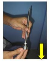
remove rotor.stator and teflon bearing
