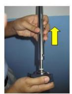
remove shaft tube and put it at a place where it cannot fall down as impact might damage it
